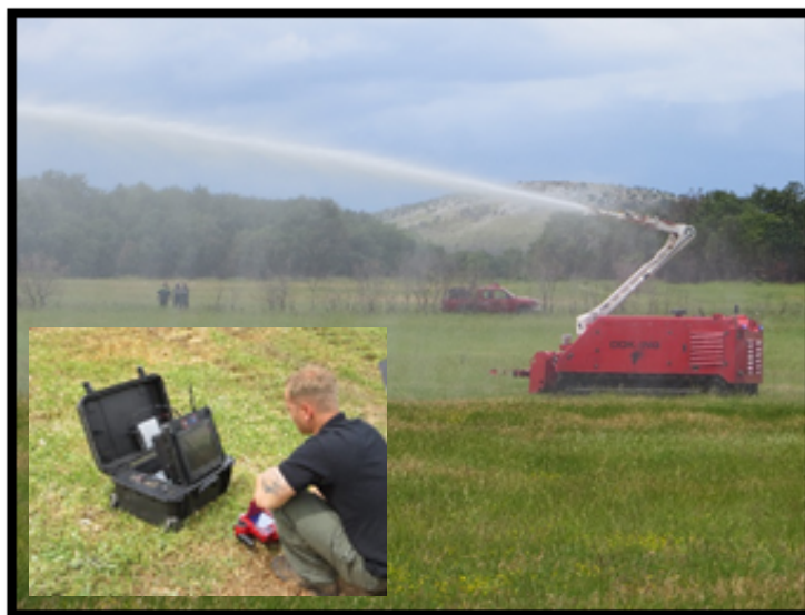
REMOTE OPERATED TRACK VEHICLE EQUIPPED WITH DOZER BLADE, HYDRAULIC JAWS AND BOOM MOUNTED WATER CANNON
